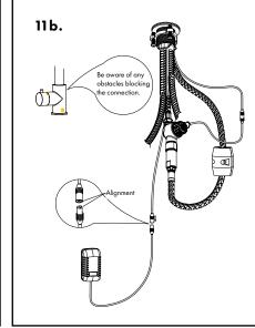
Connect the female part of the faucet Connect to the plug. to the male part of the control box.
