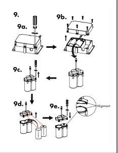
Put the batteries into the control box.
