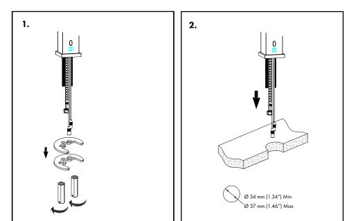
Loosen the fixing nut and screws and Mount faucet to counter top. put aside.
