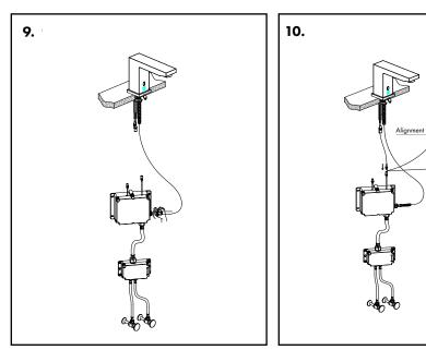
Attach the hose to the opening in the control box.
