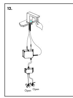
After installing the hardware and electrical components, let the system sit for at least a minute before testing the water.
