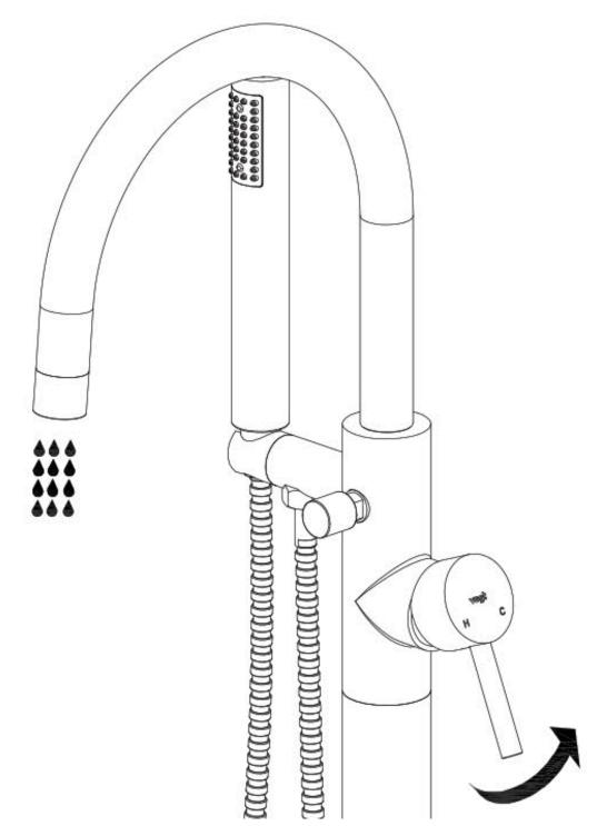
With installation now complete, turn hot and cold water lines back on to the unit, then pull water valve lever.
