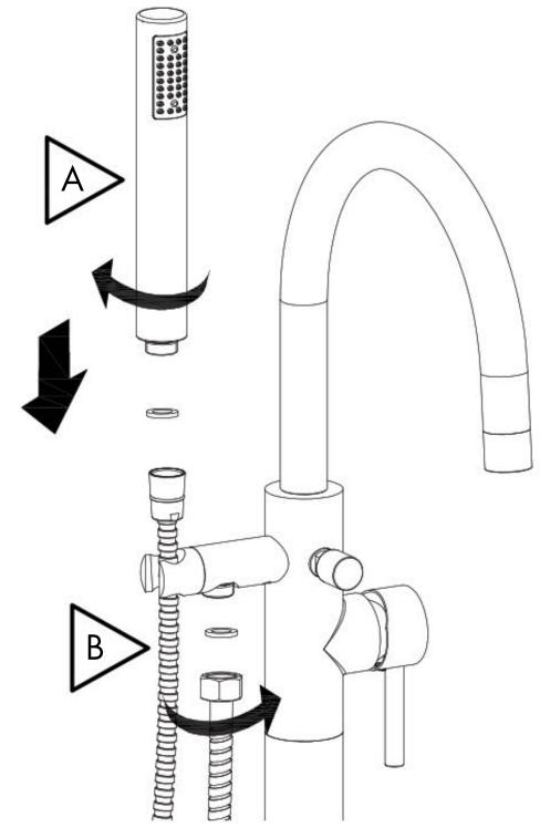
Remove plastic coverings on shower handle and shower hose and use washers to connect to main tub filler body. Use care to not overtighten.
