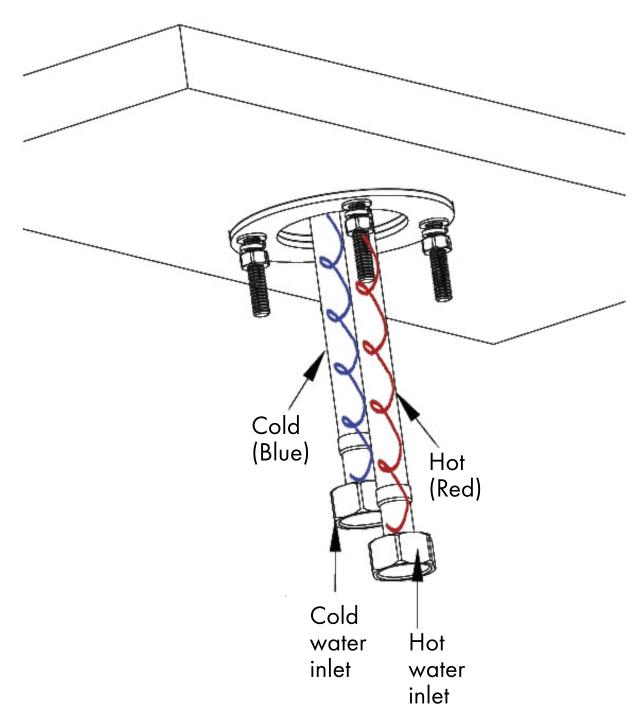
Carefully attach cold and hot water lines, ensuring connections are firm.
