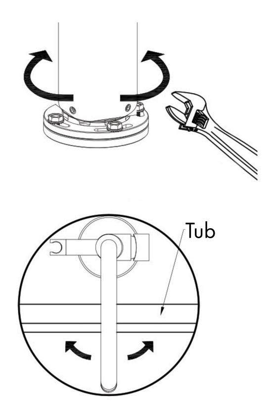
• Adjust the spout direction clockwise or counter clockwise to the proper position, then tighten bolts into place with adjustable/socket wrench.
