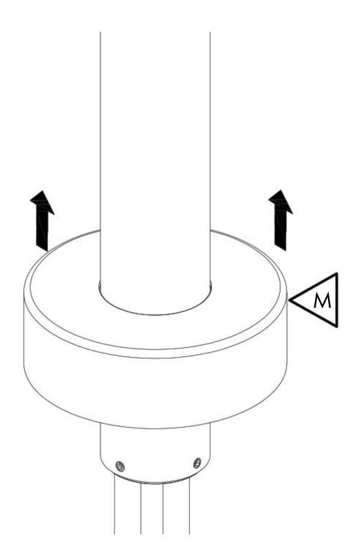
Next, on the main tub filler body, slide the mounting cap over the hot and cold water lines at the bottom and up to the base. Use caution to avoid scratching or damaging your equipment in the process.
