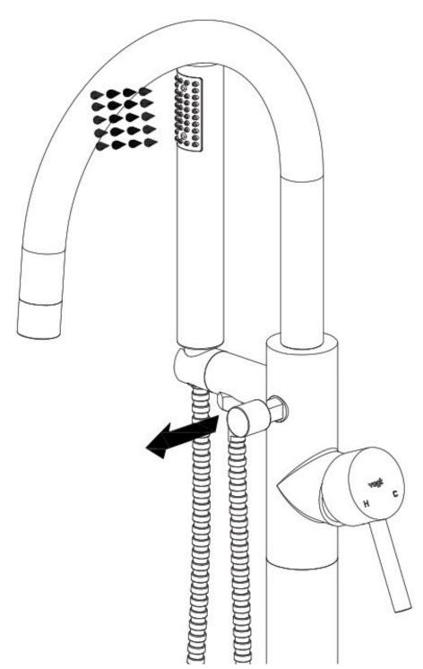
Lastly, to set the shower handle system, pull on the diverter valve knob with the water on (see arrow).
